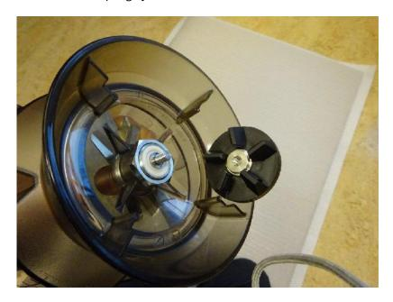
5. Using a torque wrench or a spanner, undo the nut that holds the knife unit.
