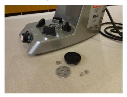
3. Remove 4 feet with screw, one center screw and bottom plate from machine.
