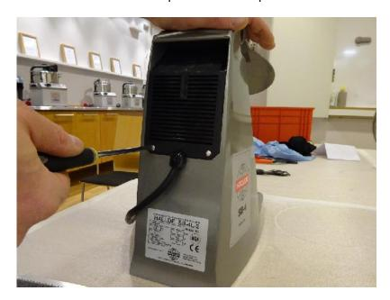
3. Turn the machine on its side and pull out the back plate and circuit board.
