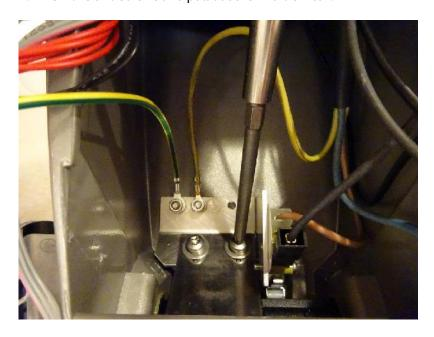
5. Install the new micro switch, be careful to position the two notches in the right position.
