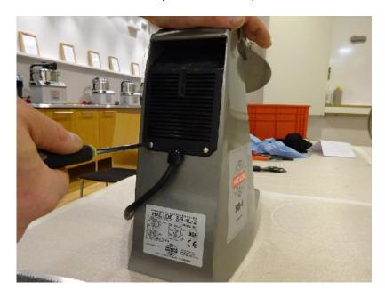
4. Turn the machine on its side, disconnect the potentiometer and pulse push buttons wires from the circuit board.
