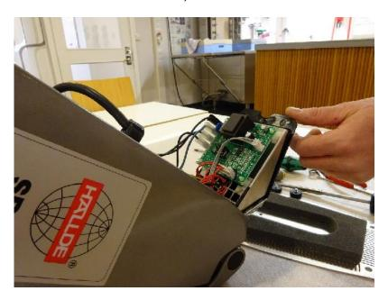
3. Disconnect the circuit board from the back plate by compressing the four quick connectors.
