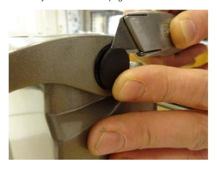
3. Carefully push the camshaft out using a screwdriver.
