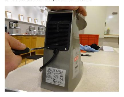
$2. \quad \text{Turn the machine on its side and pull out the back plate and circuit board.}$
