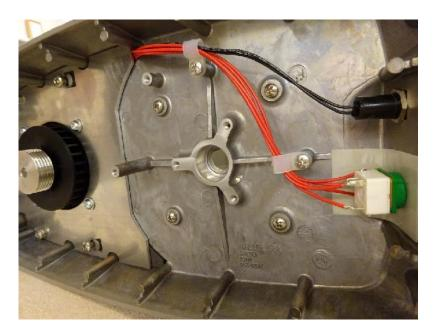
6. Install the new drive shaft and assemble in reverse order. Tighten the drive belt as described under "Motor". Use Loctite to secure the screw that holds the coupling in position.
