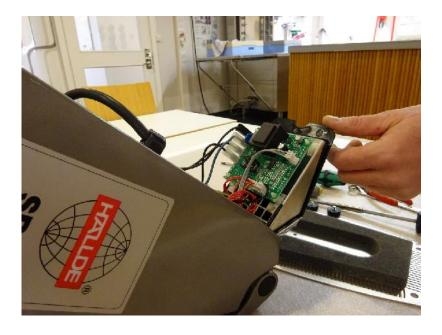
5. Open the cable clips and pull out the wires to the potentiometer and pulse push button.
