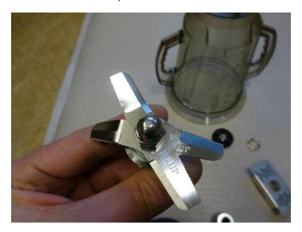
Note! Tightening torque for domed nut that holds the knifes is 10 Nm (7.4 lb ft) and tightening torque for nut that looks the knife unit to the jug is 7 Nm (5.2 lb ft).
