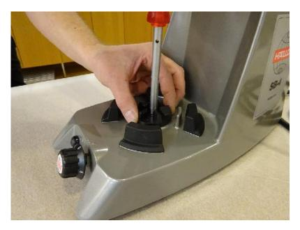
2. Remove the coupling and washer.
