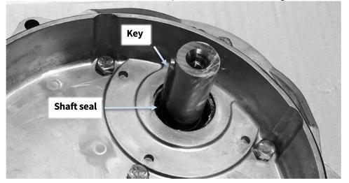
The seal is mounted from the other side and should be inserted with the spring towards the gears. Preferably it should be lubricated with the same grease as is used in the gearbox.
