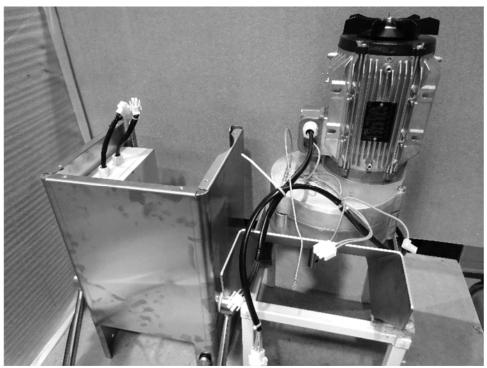
Reassemble in reversed order. The chassis fits in the slot that goes around the ejection. Inspect the gap between the chassis and knife chamber. The recommendation is to turn the 4 slotted screws so they barely touch the chassis and then have one person sitting on the unit while the 4 slotted screws are tightened. This to assure minimal gap between the knife chamber and chassis. Preferably this should be done when the machine is on its feet. Reapply some silicone to the back side if necessary.
