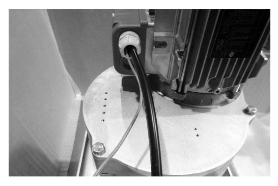
The motor is heavy and should be lifted straight up. Two persons are recommended for this step. Slightest dent on the teeth of any of the two gears will produce a knocking sound during operation. Take care not damaging the fan blades when putting the motor down.
