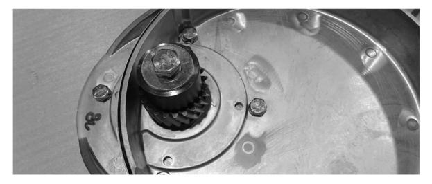
3. Remove the screw holding the gear in place on the motor shaft.
