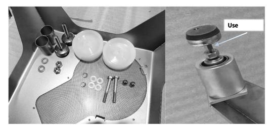
Reassemble in reversed order. The 6 screws that hold the foot is locked with a torque of ~6 Nm.
