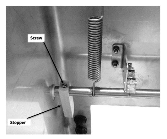
3. Undo the two screws holding the lock handle to the shaft. One on each side. The screws are locked with Loctite 243. There are two holes on each side of the shaft to which the screws align. From the inside, push the rod to one side so that it can be grabbed from the outside and pulled free. The complete lock handle can now be taken off the chassis.
