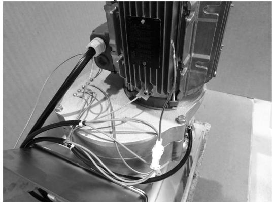
2. Remove the three hex head screws holding the gearbox together. Lift off the motor.
