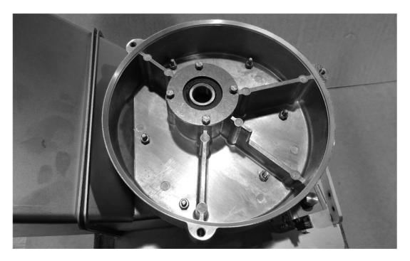
2. Bearing kit disassembled.
