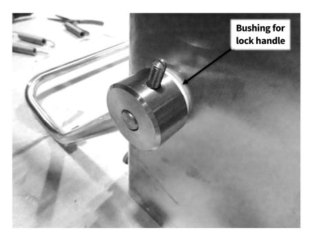
4. Disassembled locking handle.
