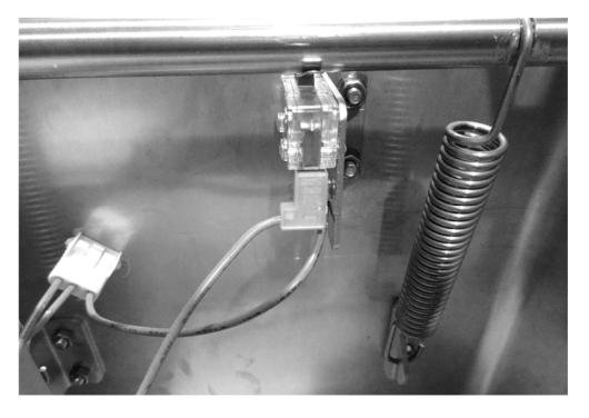
2. Remove the screw holding the stopper in place. Locked with Loctite 243. There is a hole cut out in the shaft for correct alignment of the stopper. Face the bevelled side against the chassis.
