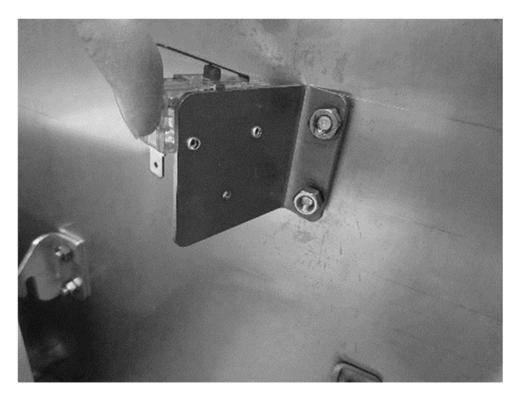
If the bracket has been moved make sure the handle (shaft) actuates the switch correctly. Assure that the contact points in the switch is clearly separated. Failure to do so could cause intermittent stops and danger to the user.
