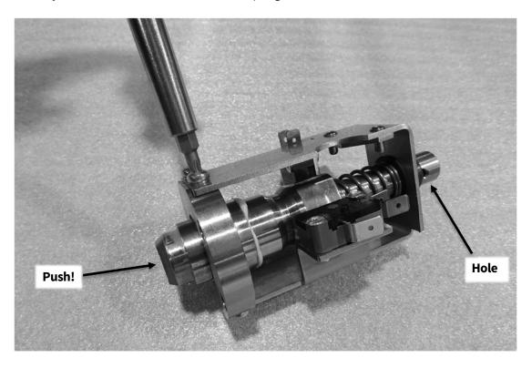
5. The micro switches are riveted to the bracket. Either replace the bracket with a complete bracket or sand down the rivets and install new micro switches. Use **aluminium** rivets or the housing of the switch will be damaged.
