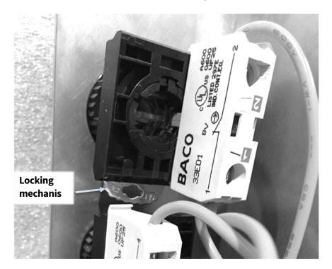
2. Undo the plastic nut holding the buttons to the chassis.
