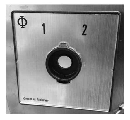
3. Remove the two screws holding the frame to the chassis. Behind the frame is a seal to prevent water from entering through the hole.
