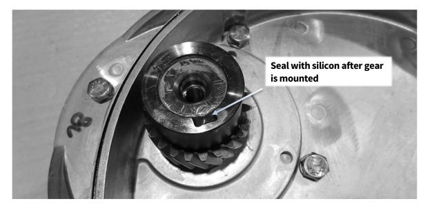
5. Remove the three hex head screws to separate the motor from the gearbox.
