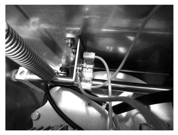
5. Undo the four slotted screws holding the chassis to the top. These are locked with Loctite 243 and a torque of 6 Nm. Use the proper tool size to avoid scratching the chassis.
