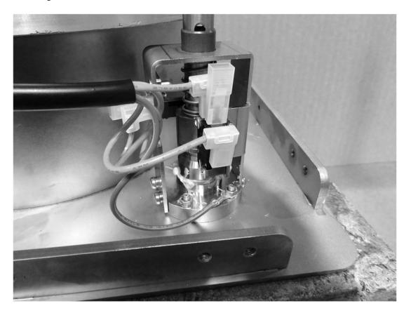
2. Remove the three nuts. Lift the unit off.
