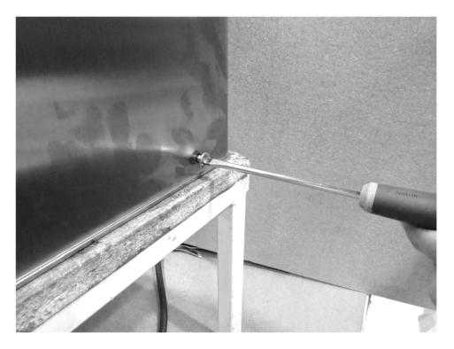
6. Make sure the wires are untangled. The chassis can now be lifted off the machine.
