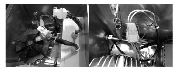
4. Unplug both wires to the micro switch. Leave the ground cable as it is.
