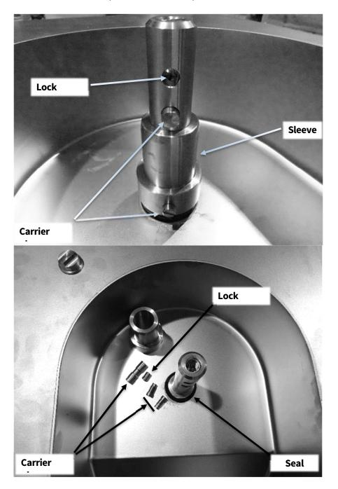
Mount the parts in reversed order. The two smaller carrier pins must be aligned with the holes in the shaft. The bigger carrier pin should be set symmetric to the shaft. The seal ring should be lubricated with food grade grease. For best result use Loctite 7649 then 2701 when refastening the screws. Leave it to harden according to recommendations in this manual. Always wipe off any excess fluid.
