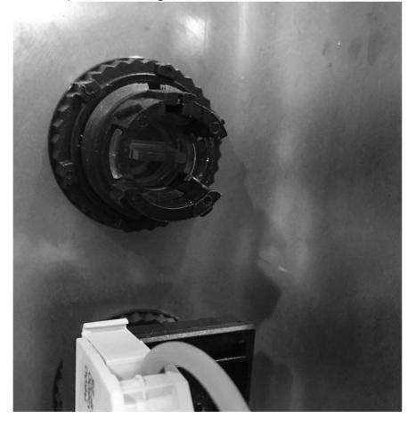
3. Press the button out of the hole. Note the cut-out in the chassis which is aligned with the small notch on the button.
