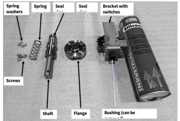
7. Completely disassembled micro switch unit.
