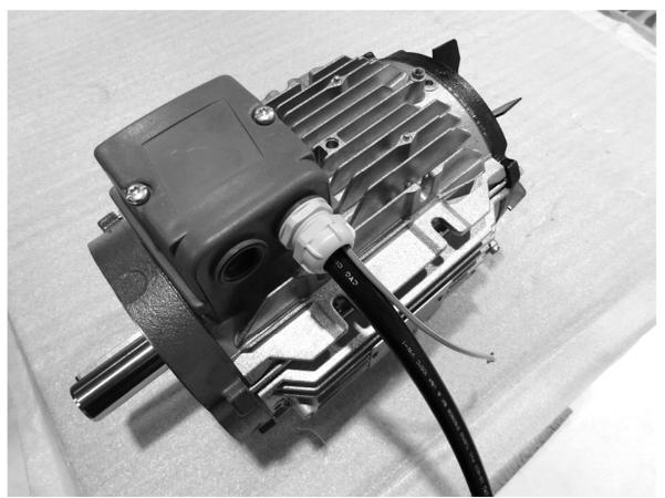
Reassemble in reversed order. Do not forget to seal the keyway with silicone on the motor once the small gear is mounted. See wiring diagram at <u>www.hallde.com</u> for internal wiring.
