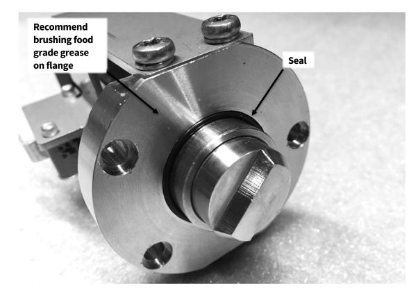
3. The flange is sealed against the knife chamber. Alternatively, silicone can be used.
