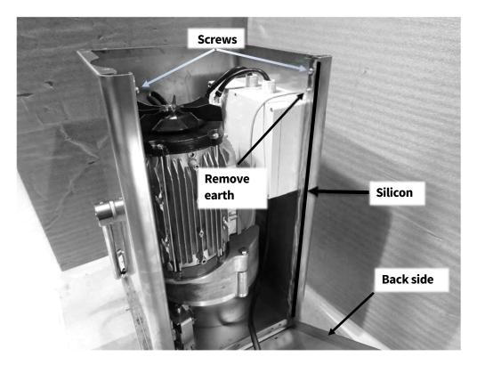
2. The back side is sealed with silicone on both sides.
