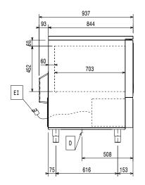
Drain Electrical inlet (power) ΕI Refrigerant Outlet
